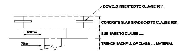
**UNREINFORCED CONCRETE SLAB**
