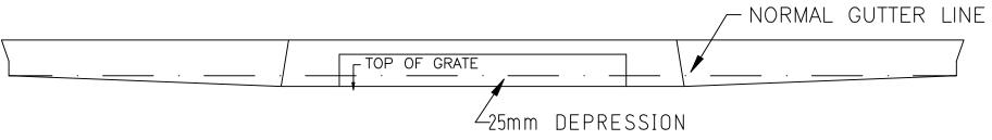
FOR CATCH BASINS IN A LINE OF CONCRETE CURBING OR GRANITE CURBING.
