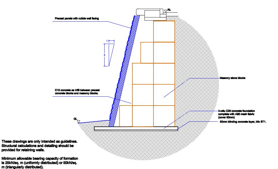
Weep holes must be provided for the draining of water behind the retaining wall.
