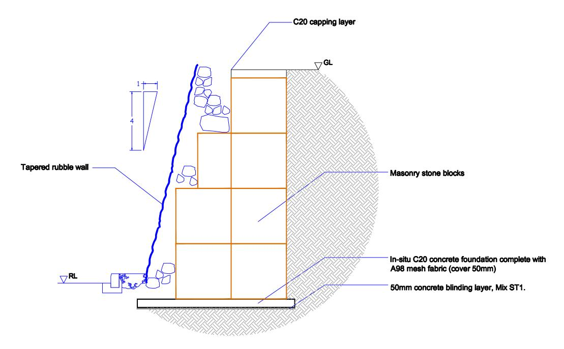
These drawings are only intended as guidelines. Structural calculations and detailing should be provided for retaining walls.
