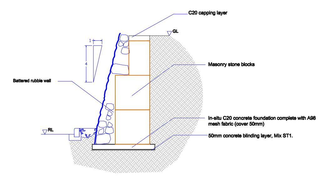
These drawings are only intended as guidelines. Structural calculations and detailing should be provided for retaining walls.
