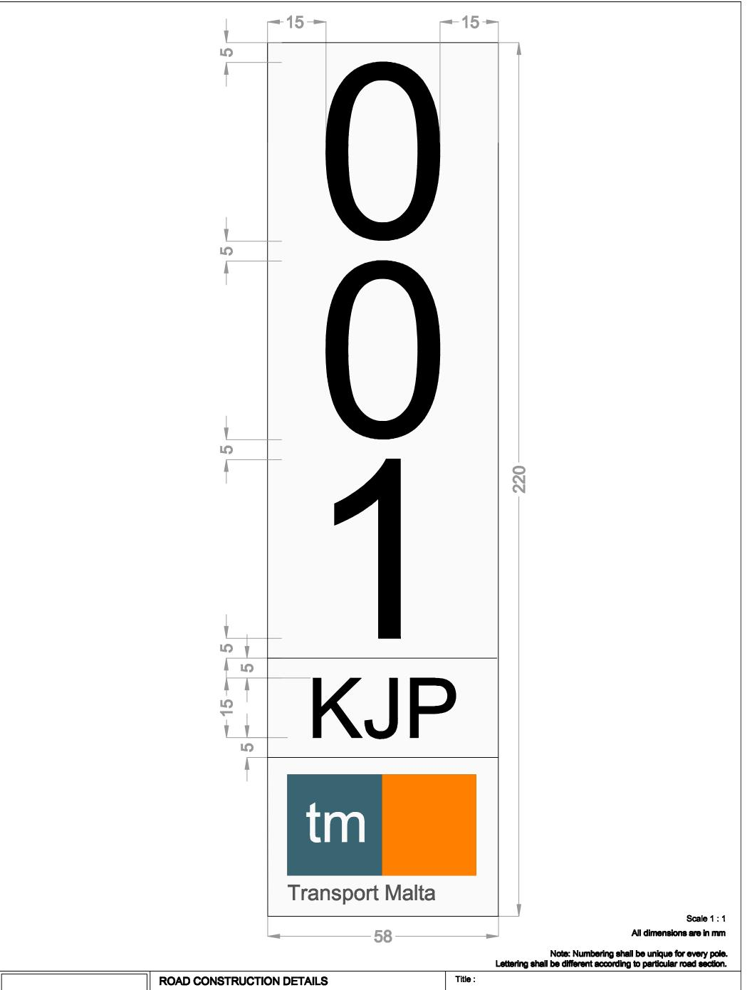
STREET LIGHT POLE LABEL SAMPLE Road Lighting Columns and Brackets Rev : Remarks : Drawn : Date : Sheet Size: E.Ç.F. Feb. 2013 Issued drawing. RCD 1300/10 **A4** E.C.F. Α Revised drawing. Apr. 2013 E.Ç.F. В Revised drawing. Nov. 2013
