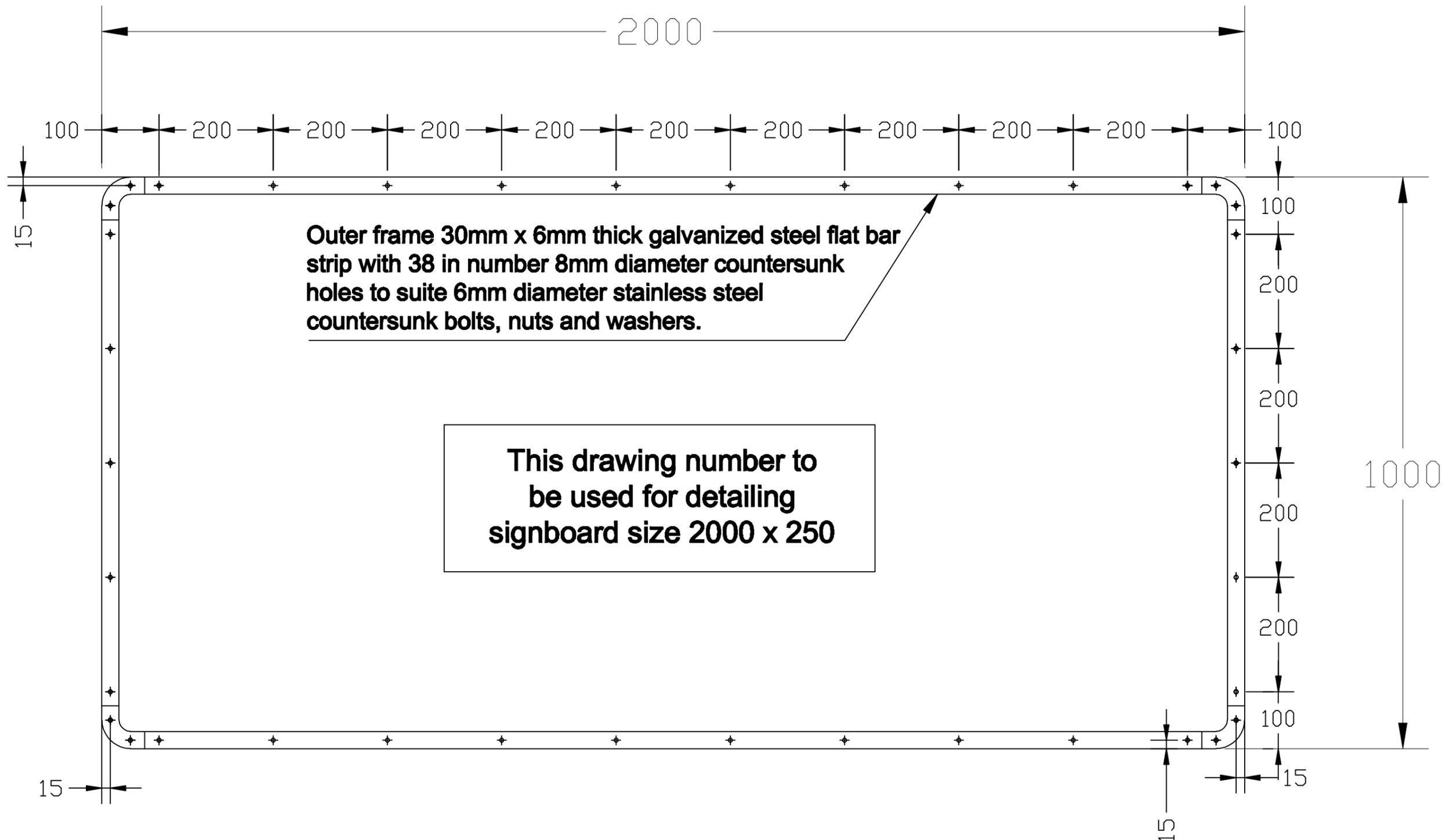
**Outer frame 30mm x 6mm thick galvanized steel flat bar strip with 38 in number 8mm diameter countersunk holes to suite 6mm diameter stainless steel countersunk bolts, nuts and washers.**
