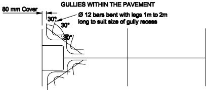
FIG. 1 JOINT WITHIN GULLY DIMENSION (Preferred position)
