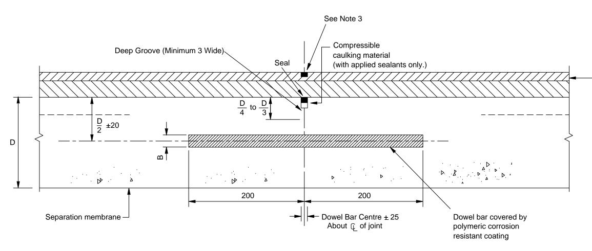
**CONTRACTION JOINT - WITH SAWN GROOVE**
