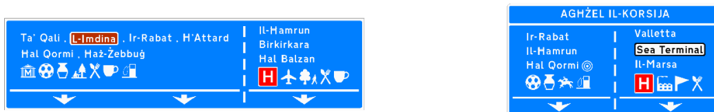
Advance Direction Signs for Dedicated Lanes to select desired Destinations for preparation of Change in direction from existing driving route.
