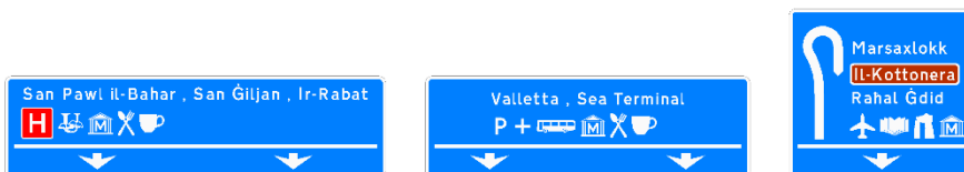
Advance Direction Signs for a 5 lane road. A combination of 2 types of signs to suit the required situation. Dedicated Lane signs and Map Type sign.
