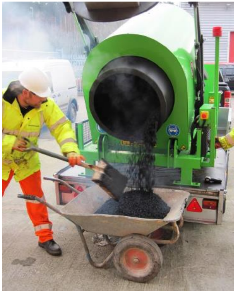
Figure 550- 7 Alternative A – Proprietary Hot Surfacing Mixer (SMA and AC) (Illustrative Only – Source Roadmender (UK))
